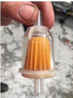
So I had a filter that was blocked by a contaminant that was invisible to the eye. The contaminant was able to flow through the brass gauze filter on the taps but was slowly blocking the finer paper element filter.
