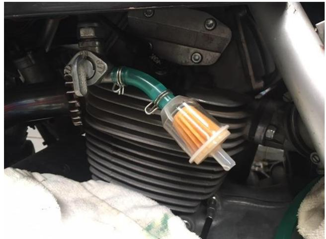
I reinstalled the fuel tap and connected up the fuel lines. With the rear bowl off I still had no fuel flow to the rear carburettor. I pulled out the needle from the needle and seat. Still no fuel flow. I then removed the banjo fitting from the carburettor, and still no flow. I decided to work my way back to the tank.
